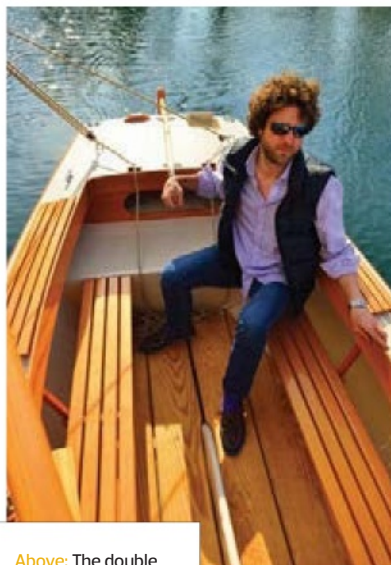
Above: The double ended mainsheet can be trimmed on either tack without a traveller
